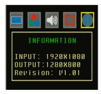
Displaying both input source and output display timing with software firmware version.
