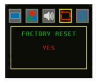
Select YES to return to the factory setting. Factory setting on display is at 1280 x 720p @60Hz with full size screen, Color setting are as the bracket in the OSD chart and SDI audio is on auto.
