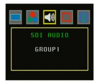
Select SDI audio output from 4 different group and each group contents 2CH or from auto which contain up to 7.1Ch follow by input source signal. If no audio output is require the audio can also be mute by selecting off.
